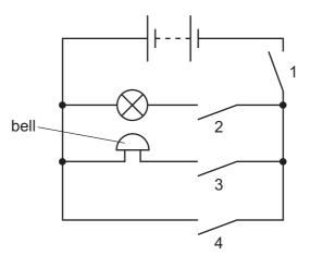
Which switches must be closed for the bell to ring without lighting the lamp?
