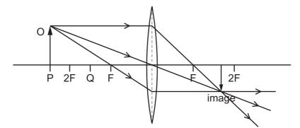
The object O is moved to point Q on the diagram.
