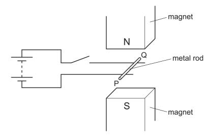
When the switch is closed, the rod moves to the right.
