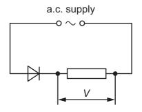
Which graph shows how the potential difference V across the resistor varies with time t?
