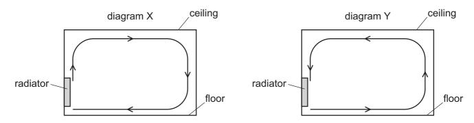
Which diagram and reason explain the heating of the room by convection?
